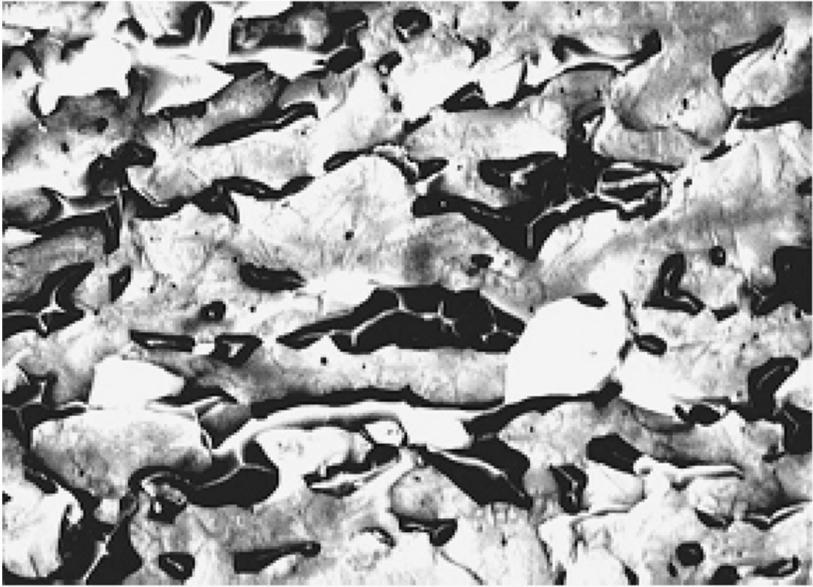
Figure 14 Example of fracture surface showing \text{Al}_2\text{O}_3 and Al phases interpenetrated.
